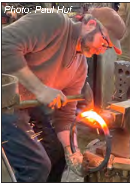
Forming and welding the outer ring.
