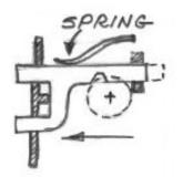
Double bolts are actually a single bolt as shown. Make your layout carefully to be sure there is room for all the parts.
