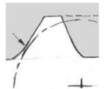
To prevent the problem above the notch should have a gentle curve at the bottom. When the key passed the curve there is significant clearance. If the bolt should slide back a little the key can push it out of the way easily.
