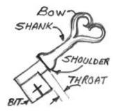
The parts of a key are the bow (handle), shank, shoulder, throat and bit. The shoulder is optional depending on the type of key. Most barrel keys do not need a shoulder but may have one for decorative purposes. Modern bit keys that work from both sides of a lock need a shoulder to position the bit in the lock.
