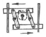
Two directional bolts generally use simple lever mechanisms. However from this point onwards locks can have gears, racks and all sorts of mechanical devices that we are not going to get into.
