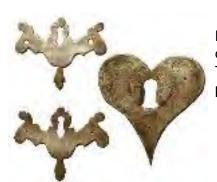
Lock making opened up other areas of hardware to supply. These are replacement drawer pull plates and matching lock plate I made for an 18th century dower chest. The original pull plates had all the little tabs that stick out broken off and heart lock plate was missing. Its shape was determined from the bleaching of the wood.
